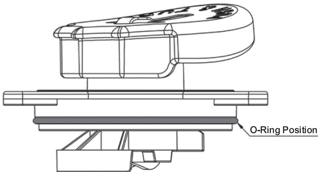
**EN:** TO REPLACE THE VALVE, UNSCREW THE THREE SCREWS AROUND IT. REMOVE ALL COMPONENTS OF THE OLD VALVE AND GREASE THE INTERNAL EDGE OF THE SEAT WITH THE SUPPLIED GREASE.
